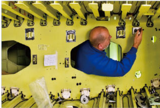
General Assembly Line for the Wing of A320 Airbus
