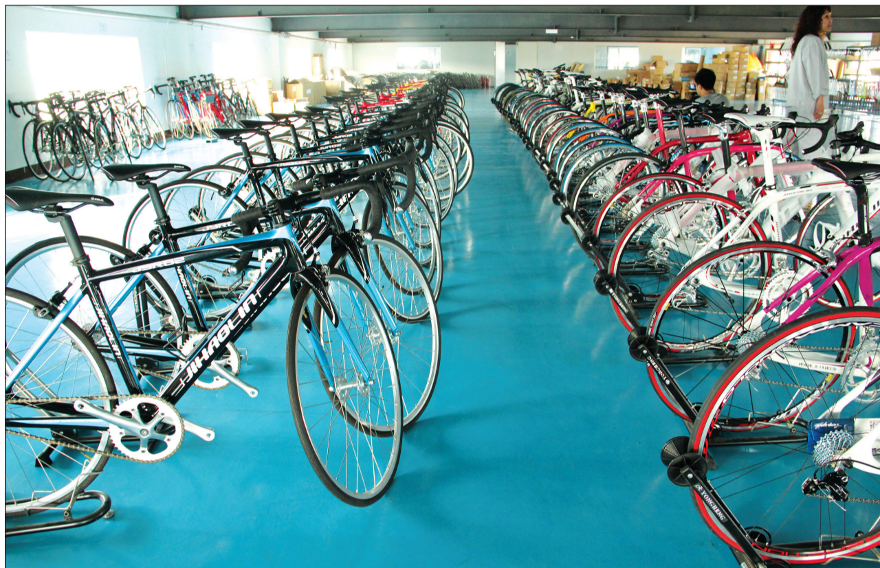
Rows of bicycles made of carbon fiber in Jilin Jiyan High-tech Fiber Co Ltd. The bicycles on average weigh only 3.5 to 4.5 kilograms thanks to the application of the new materials.
